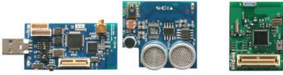
(a) MPS430 H-mote (b) Sensor board (c) CC2430 H-mote
