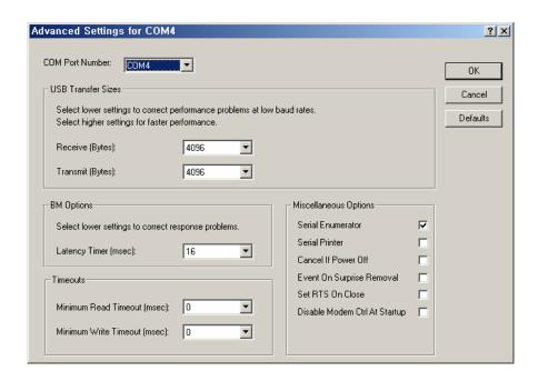
[Caution] Cygwin released before Oct. 2006 is compiled to recognize maximum 15 serial devices. Virtual COM ports should be mapped to COM1 to COM15 since the RETOS application installation tool injector uses the Cygwin standard library.
