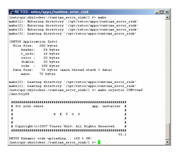
To detect run-time errors of the application, a host PC with a connected sink mote is required. (Install app/runtime\_error\_sink application into this mote.) The sink mote receives and reports the error reported from the remote sensor mote.
