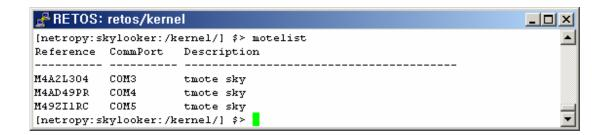
You can check if each mote is connected by typing "motelist" command.
