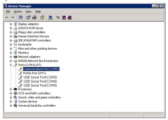
In this figure, three motes are connected to COM3, COM4 and COM5, respectively. This Virtual COM Port allows several motes to connect to the host PC and work simultaneously. Port numbers can be modified by changing COM Port Number at Port Setting > Advanced, and you can see the port number changed after reconnecting the mote of which you just changed the port number.
