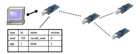
The sink mote is connected to a host PC through COM port (USB). The RETOS kernel and the code dissemination module (recode\_mod) are installed on every sensor mote including the sink mote. Each mote in the network shares the application list and the version information together. Since the host PC installs an application into the sink mote, every mote in the network communicates with each other and installs the application. In that way, every sensor mote has
