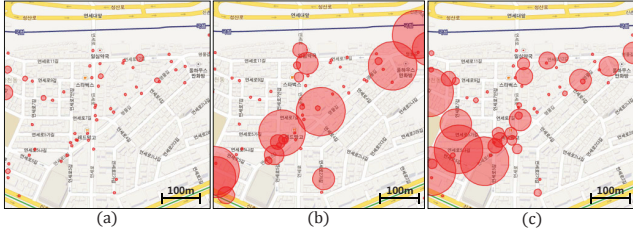
Figure 10. Distribution of visited food places and nightlife places in 600 m x 550 m region. The circles are places and the size of the circle indicates the number of visitors; (a) without packet sensing during the entire day, (b) 11 am to 2 pm with packet sensing, and (c) 5 pm to 11 pm with packet sensing. Our methods estimated rich dynamics of urban mobility according to time-of-day.
