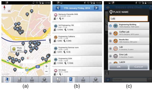
Figure 5. User interface of smartphone application. The application displays a user’s mobility on (a) the Google map and (b) the list. (c) The user annotates the place name along with the list of places in Facebook.
