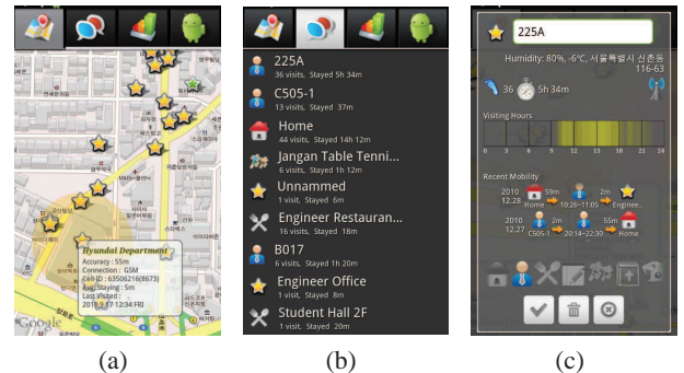
Figure 6. User interface of SmartDC. The application displays a user's meaningful places on (a) the Google map, and (b) the list. It also visualizes (c) place information, including place name, connectivity, residence-time, and mobility history. The application called LifeMap is available in Android Market.
