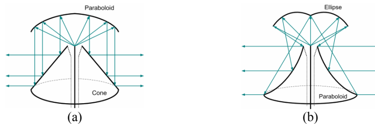
Fig. 16. Schematic diagram and radiation direction on side view of dual reflector omni-directional antenna consisting of (a) a paraboloid and a cone [22], and (b) an ellipse and a paraboloid [23].
