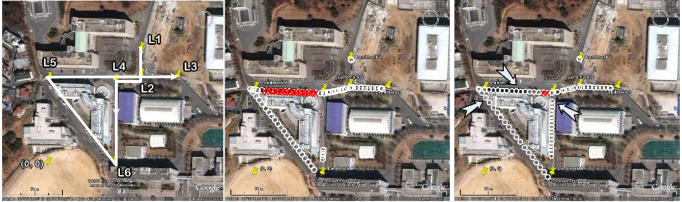
(a) Trajectory of target mobile node (b) Result with 6 landmarks (c) Result with 6 landmarks and 3 mobile nodes Figure 6: Location estimation results in large scale experiments
