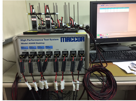
Figure 10: Experiment settings for cycling tests with Maccor 4300K.
